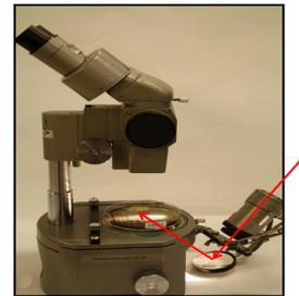
Fig.3 Binocular stereomicroscope
