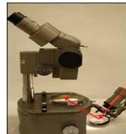
Fig.2 Binocular stereomicroscope
